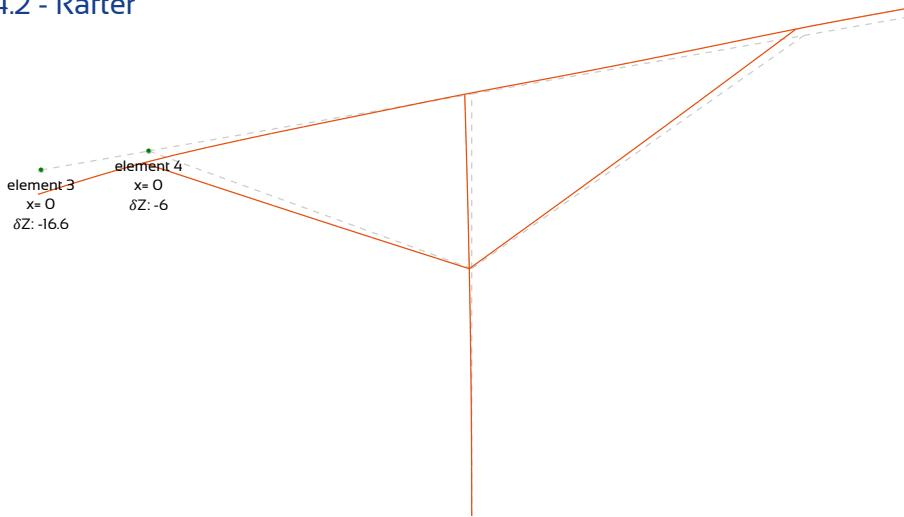
Maximum total deflection on the left side :  $\delta Z = -16.6 \text{ mm} (\text{SLS I2}) < L/100 = 49.5 \text{ mm}$
